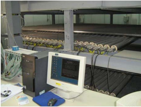
Fig. 4 Mt. Norikura muon telescope in Japan. In background: the proportional counter tubes. In foreground on the left side is the electronic box. Identical items are also used in MuSTAnG, NST, HST, SMST and KPC.
