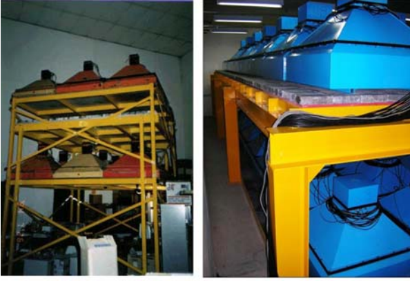
Fig. 3 Left: HST in Tasmania. Right: SMST in Brazil. In both images the lead layer between the pyramid like box with a quadratic box on top for the PMT are visible.
