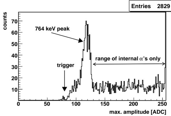
Fig. 3. Registered distribution of amplitudes of signals. Sum of 16  $^3\text{He}$  counters, 7 days of underground exposure with ‘line’ setup.
