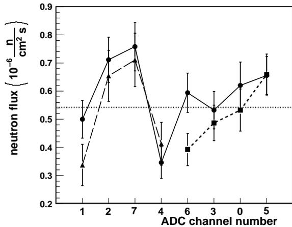
Fig. 6. Average neutron flux (horizontal dotted line) and flux values obtained from simulations and measurements for separate counter pairs for layout 'line' (dots), inner circle (triangles), and for outer circle (squares) in 'circles' layout. Indicated errors are statistical, only.
