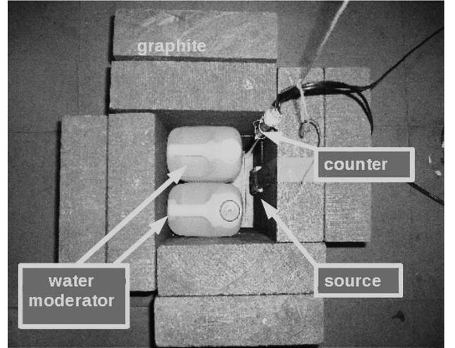
Fig. 5. Experimental setup for verifying the accuracy of simulations. Tested counter was placed inside a graphite chamber (20 cm thick wall) together with the AmBe neutron source and water moderator (20 l). Measurement was reconstructed by Monte Carlo simulation with 98% agreement.
