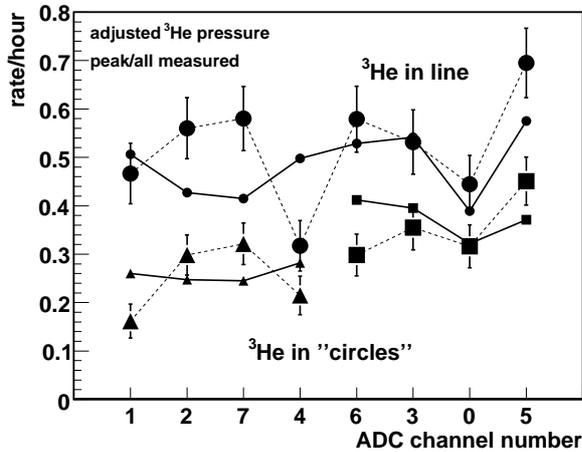
Fig. 4. Measured (dotted line) and simulated (solid line) rate of neutrons for all pairs of counters. Circles mark ‘line’ layout, triangles – ‘inner circle’, squares – ‘outer circle’. Only neutrons from 764 keV peak are counted. Simulation were normalized to the thermal neutron flux equal to  $5.42 \cdot 10^{-7} \text{ n}/(\text{cm}^2 \cdot \text{s})$ .
