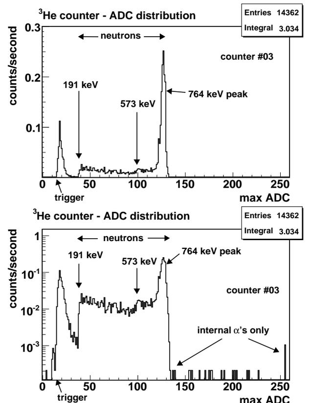
Fig. 2. Distribution of amplitudes of signals from <sup>3</sup>He counter in linear and logarithmic scale (test run with AmBe neutron source).
