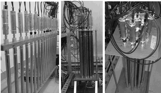
Fig. 1. Photos of detectors. Left photo shows ‘line’ setup. Center and right photos show the compact ‘circles’ layout.
