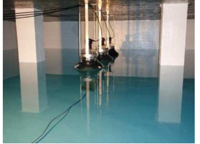
Fig. 11. Inside of a water cell of the prototype muon detector equipped with three 20 inch PMTs in an area of 52 m 2 .
