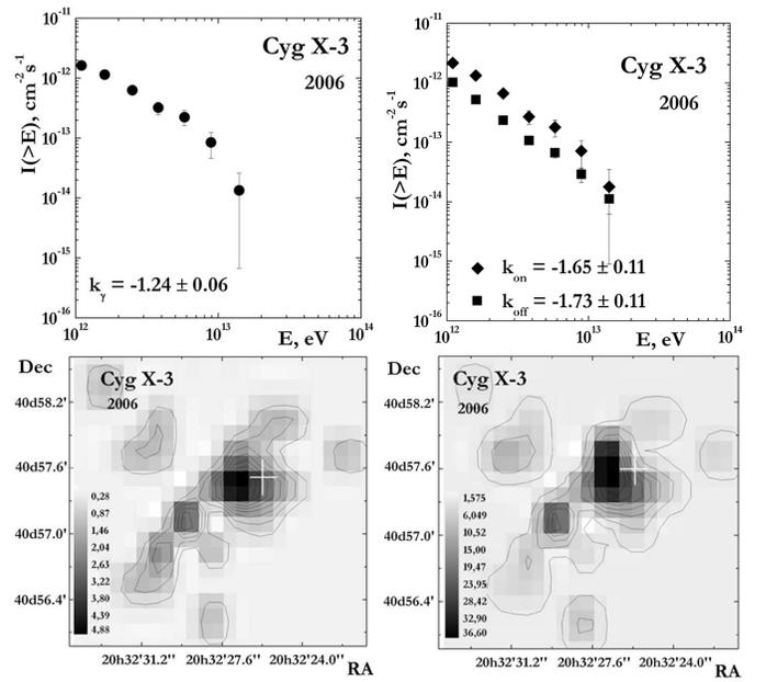
Fig. 6. **Top, left:** The Cygnus X-3 gamma-quantum spectrum in 2006 with power index of  $k_\gamma = -1.24 \pm 0.06$ ; **right:** The event spectrum from Cygnus X-3 with background  $k_{ON} = -1.65 \pm 0.11$  and spectrum of background events observed simultaneously with Cygnus X-3 -  $k_{OFF} = -1.73 \pm 0.11$ ; **Bottom, left:** The image of gamma-ray emission from Cygnus X-3 in 2006; **right:** The energy image of Cygnus X-3 (in TeV units) in 2006 by SHALON.
