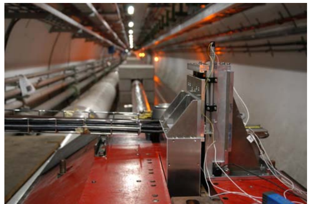
Figure 10. The LHCf detector located at the TAN, 140m away from the intersection point IP1.
