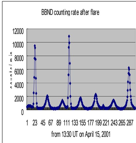
Figure 2a. The two sharp peaks at 175 and 262 were caused by the South Atlantic Anomaly. After the arrival of high energy solar particles ( after 204), the intensity of neutrons increased when the ISS approached polar regions.
