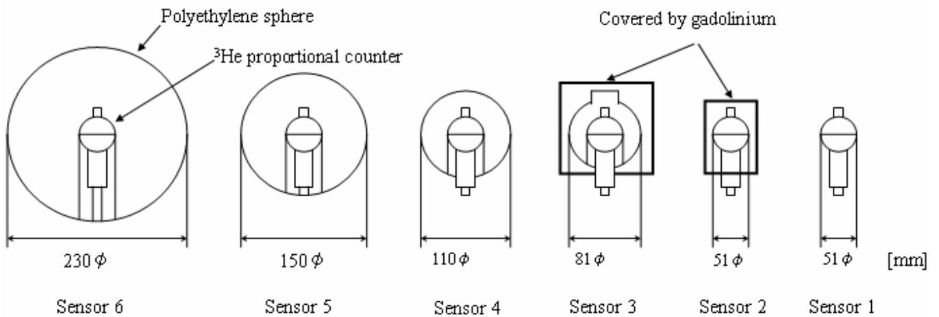
Figure 1. The six Bonner Ball Neutron Detectors were launched on the International Space Station. The sensor S6 is the largest detector, with the highest sensitivity to neutrons, at around 2 MeV. Its sensitivity extends almost uniformly throughout the energy range of 0.2–10 MeV.
