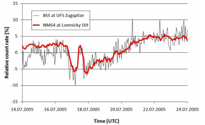
Fig. 3: Total relative hourly count rates obtained by the BSS system on the UFS in July 2005 (thin line) [7] compared to those measured by the NM at Lomnický Stit (thick line) [16].
