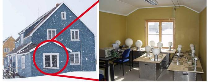
Fig. 2: One-floor extension of the Koldewey station of the AWI (left) in Ny-Ålesund, Spitsbergen, and Bonner sphere spectrometer inside the extension (right).
