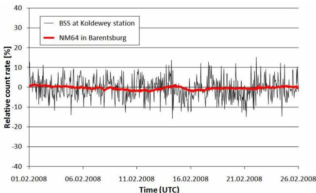
Fig. 5: Total relative hourly count rates of the BSS at the Koldewey station in February 2008 (thin line) and relative count rate of the NM in Barentsburg (thick line) [18]; data are normalized to the corresponding mean values in this period of time.
