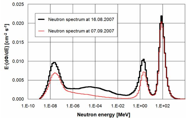
Fig. 4: Unfolded neutron spectra measured at the UFS on 16<sup>th</sup> August 2007 (dry and sunny weather), and three weeks later on 7<sup>th</sup> September 2007 with heavy snow fall and about 1.5 m snow cover on the terrace.
